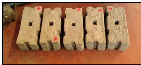
Figure 1: Finished Interlocking Block
